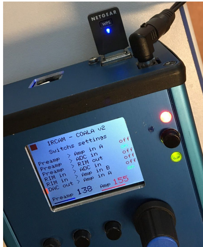
Fig.5: The Coala v2: screen controls and Wifi dongle
