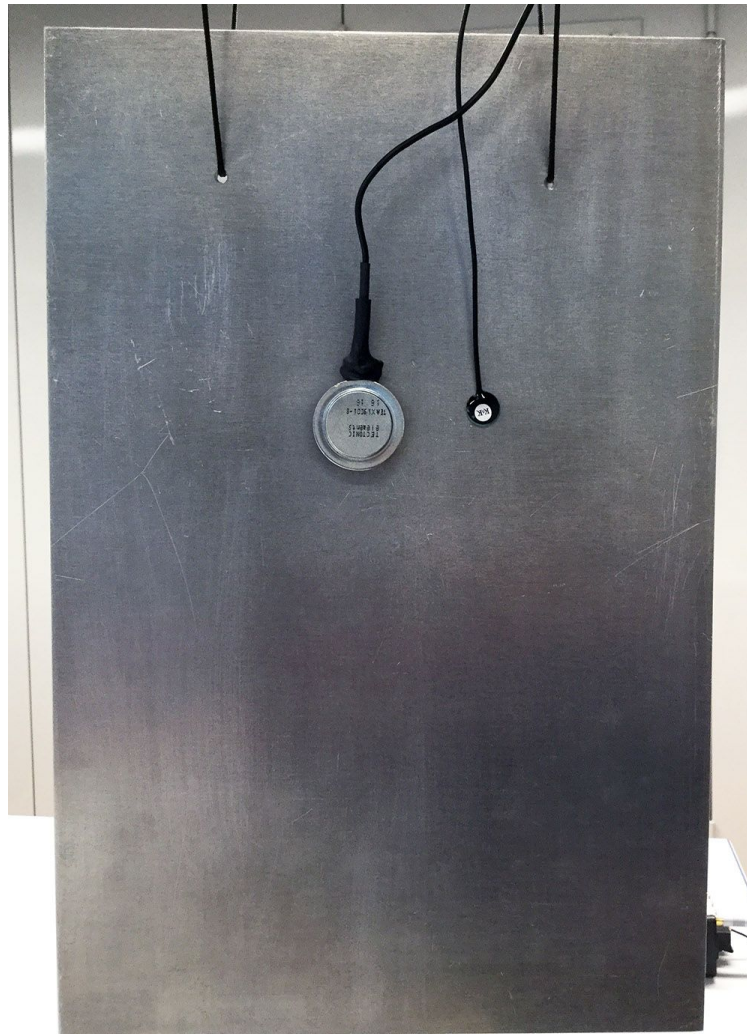
Fig.6: The steel plate equipped with a sensor (piezo) and an actuator.
