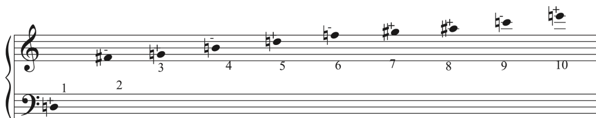
Fig. 11: The note sequence of the partial frequencies identified on the resonating structure.
